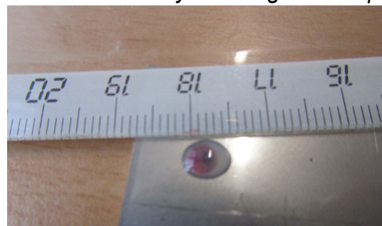
Clear Red colouring: 2% Mo. Stainless steel AISI 316 group.
