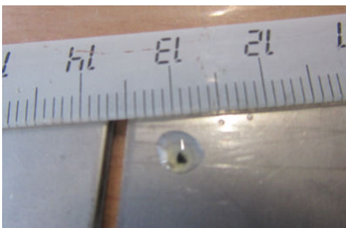
No red colouring: <05% Mo. Stainless steel AISI 304 group.
