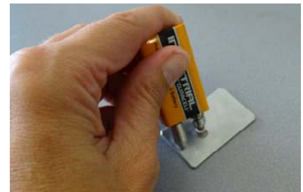
Lift the short pin in the drip during 1 second, while leaving the long pin on the surface for making a circuit.
