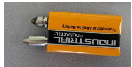
MolyTester XS with the long pin (the anode, +) and the short pin (the cathode, -)
